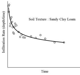
Figure 2. Infiltration rate
