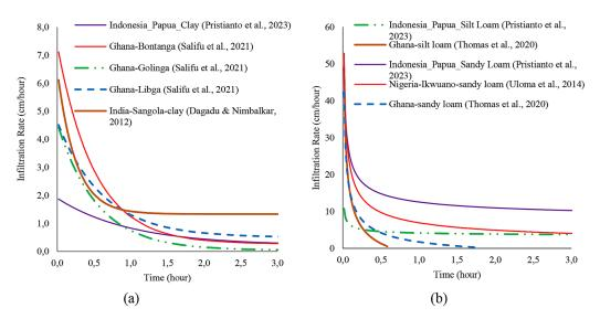
**Figure 4.** Comparison of the theoretical lines of Horton model (a), and Philip's model (b), with model parameters from research results in Indonesia, Ghana, Nigeria and India
